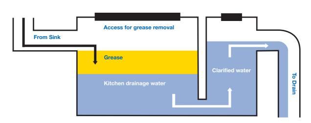
Diagram of an "under-the-sink" grease trap
